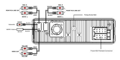
Note: Use the clip end of a Ground Line provided by manufacturer to connect the Fixing Screw Bolt, use another end of the Ground Line to connect the negative pole of the power source. Otherwise, the video on screen maybe flashes.
